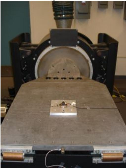
The table essentially uses a large stereo speaker in the circular area at the back of this image to vibrate the table on a layer of oil using a pre-programmed vibration profile.
